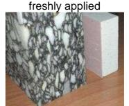
The glue layer was always applied over the full surface on one side using a paint roller.
