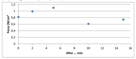
After the glue is freshly applied onto one side and if the 'open dry' waiting time is below 15 minutes before pressing the 2 layers against each other the glue can withstand a tensile stress of at least 0.61 N/cm<sup>2</sup> (= 6.1 kPa or  $\approx$  622 kg/m<sup>2</sup>).
