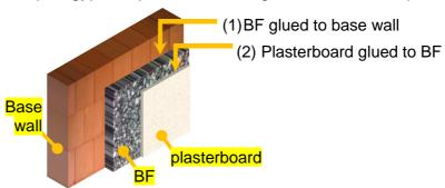
Doing so a good performing mass-spring system is realized. The base wall (or ceiling) could be of any type of common building material. Instead of the gypsum plasterboard also other types of building panels could be used.
