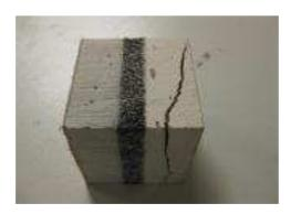
Initial tack This testing resulted in tensile stress values between 0.61 and 1.1 N/cm<sup>2</sup> (depending on the 'open dry time'). The maximum StDev was 0.54 N/cm<sup>2</sup>.
