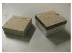
Sample 2: frature between foam and plaster board
